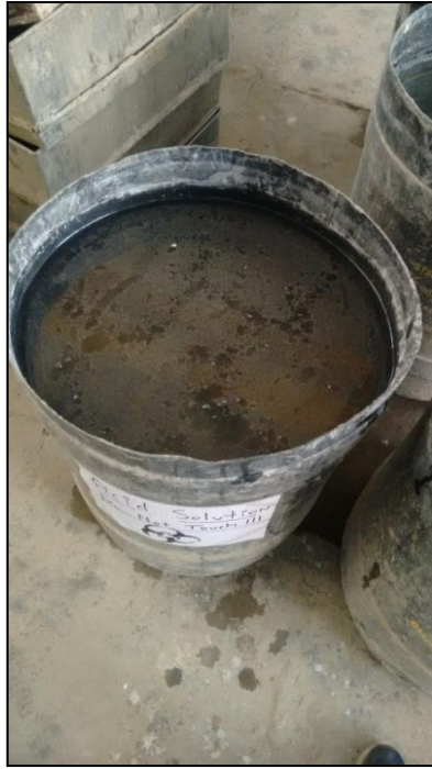
Fig 1: Cubes immersed in the acid solution
