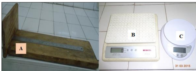
Fig 2: Fish measuring and weighing equipment: A = ichthyometer; B = EKS Electronic scale and C = WH-B05 Series Electronic Kitchen Scale User's Manual scale)
