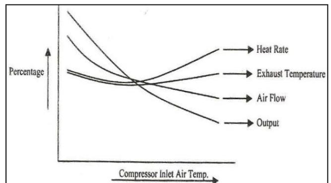
**Fig 4:** Effect of air temperature on gas turbine performance heat rate, airflow and turbine exhaust temperature the total gain in combined cycle power output due to reduction of inlet air temperature is higher than a gas turbine running in simple cycle mode.
