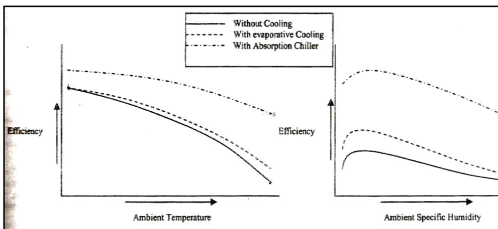
**Fig 5:** Efficiency v/s temperature and also with ambient specific humidity
