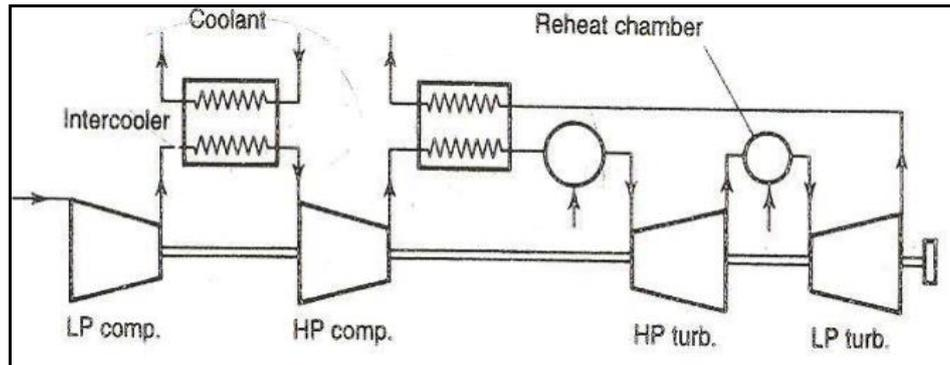
Fig 6: Integrated plant with inter, heat exchange, reheat.
