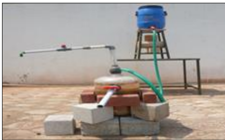
Fig 3: UASB reactor before production of biogas
