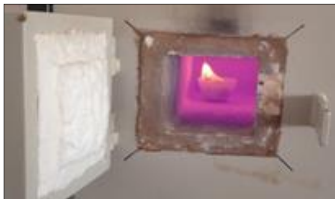
Fig 9: Burning residues in oven for sulphate test
