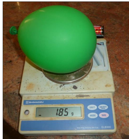
Fig 6: Weight of the ballon with bio-gas
