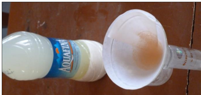
Fig 8: Filtrating sample for sulphate test
