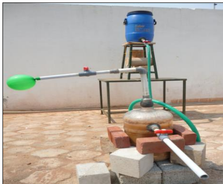
Fig 4: UASB reactor after production of biogas
