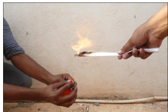
Fig 7: Burning of bio-gas filled in the ballon
