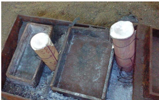
Fig 1: Mould and cast product after casting
