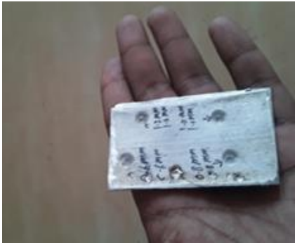
Fig 2: Test pieces (After Spot welding)
