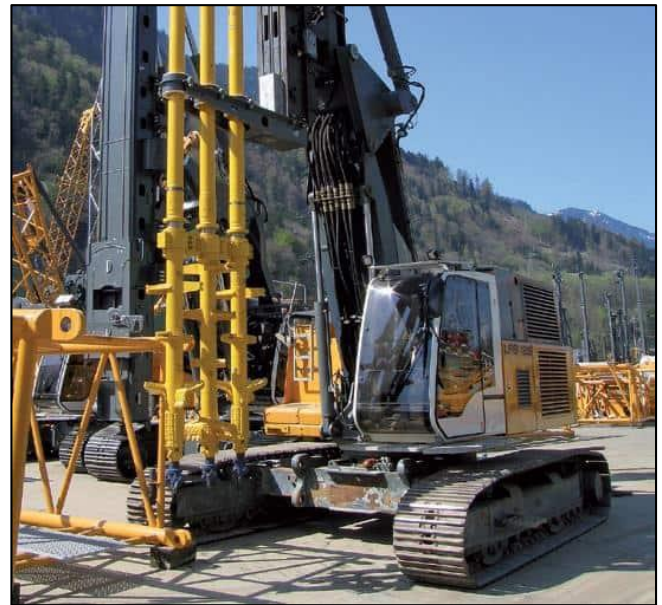
Fig 2: Deep soil mixing rig with triple mixing tool
