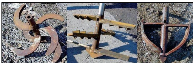
Fig 1: A selection of dry mixing tools used for different soils
