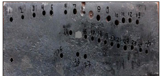
Fig 1: Specimen after EDM drilling
