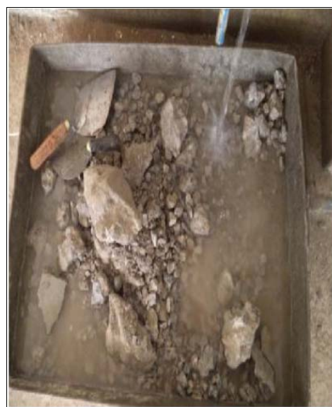
Fig 1: Crushing and washing of recycled aggregates
