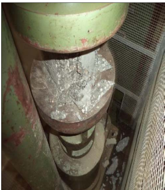
Fig 3: Compression test on cubes
