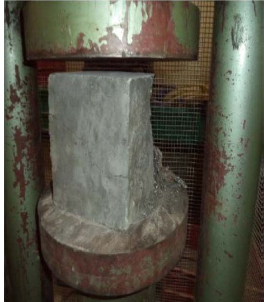
Fig 4: Crushed specimen after compression test
